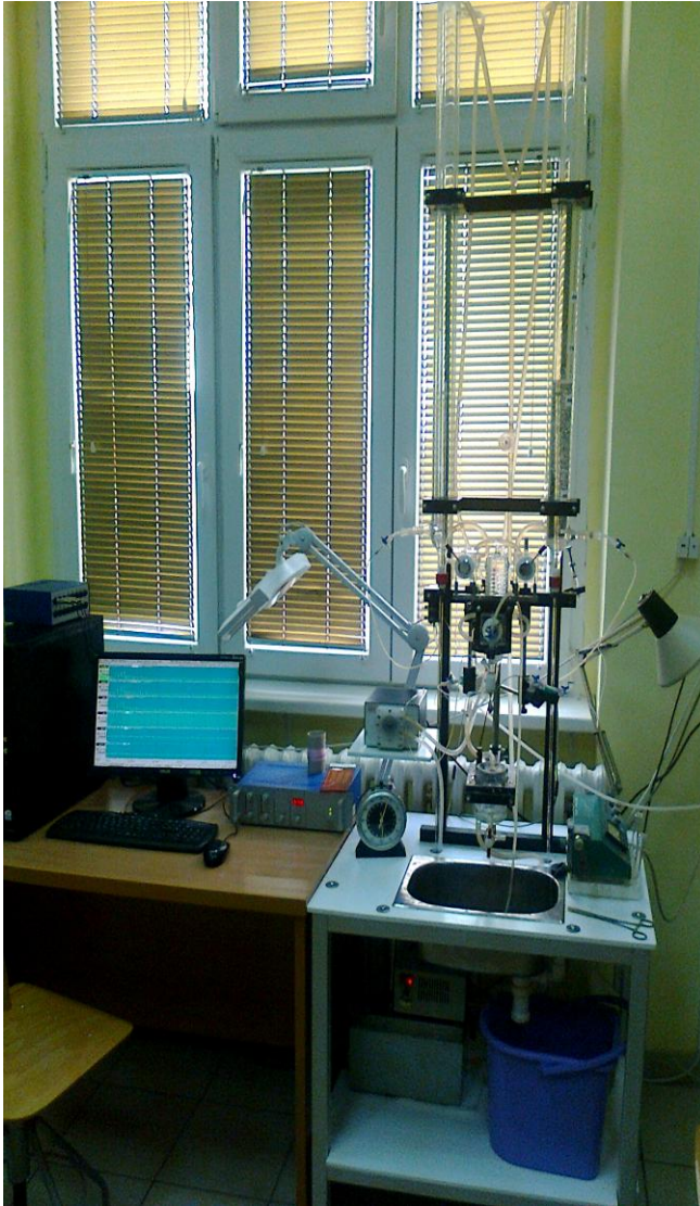
Слика 1. Модификовани апарат по Langendorff-у (LF-11-LF01 F-P, Perfusion systems for isolated, small mammalian hearts according to Langendorff, Experimtria LTD Budapest, Hungary)
